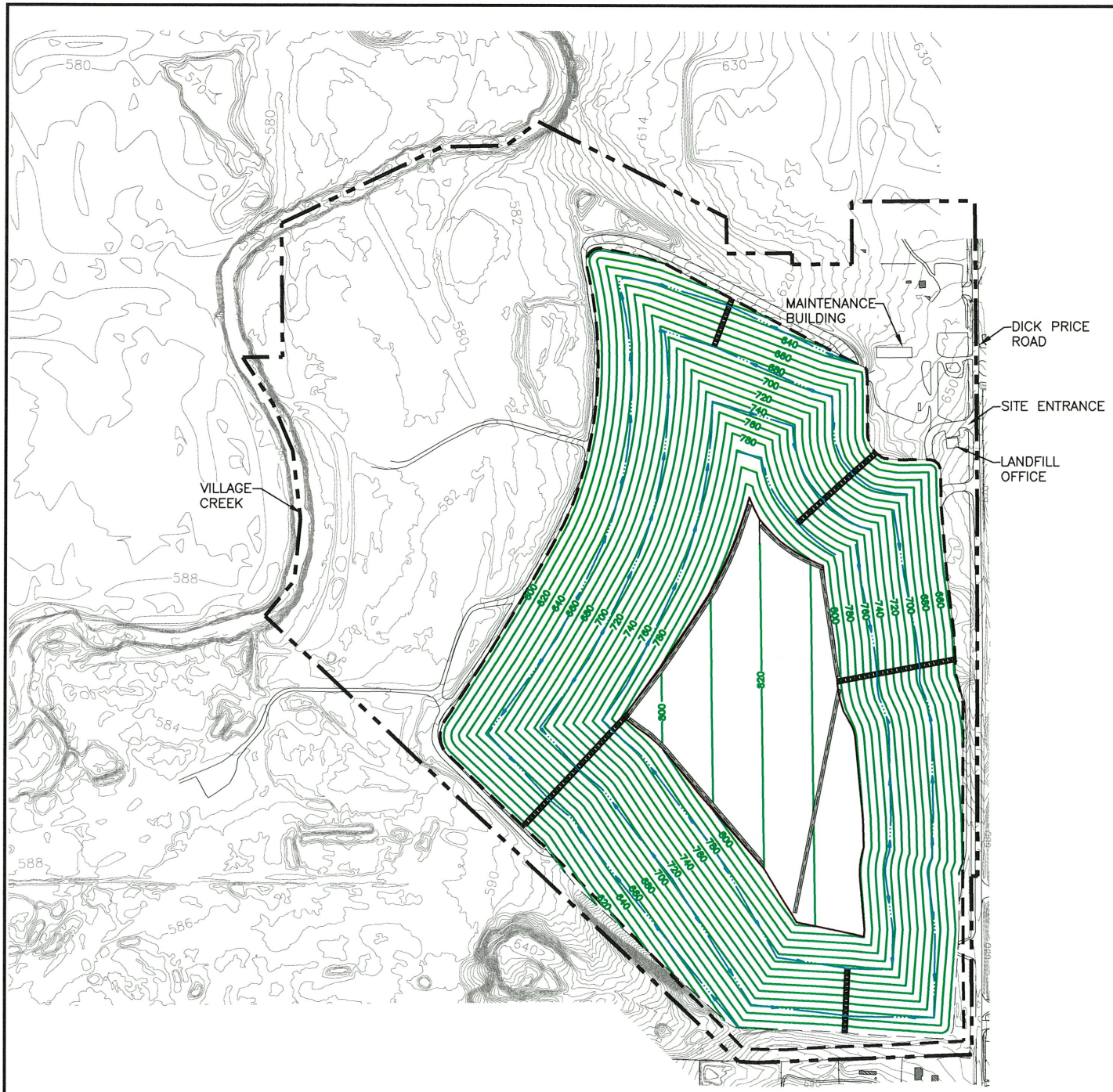
PERMITTED LANDFILL COMPLETION PLAN
