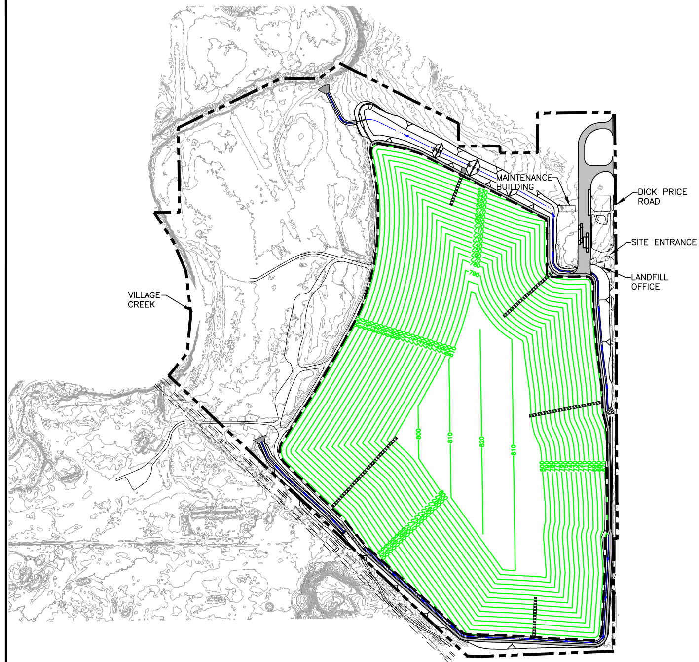
PERMITTED LANDFILL COMPLETION PLAN
