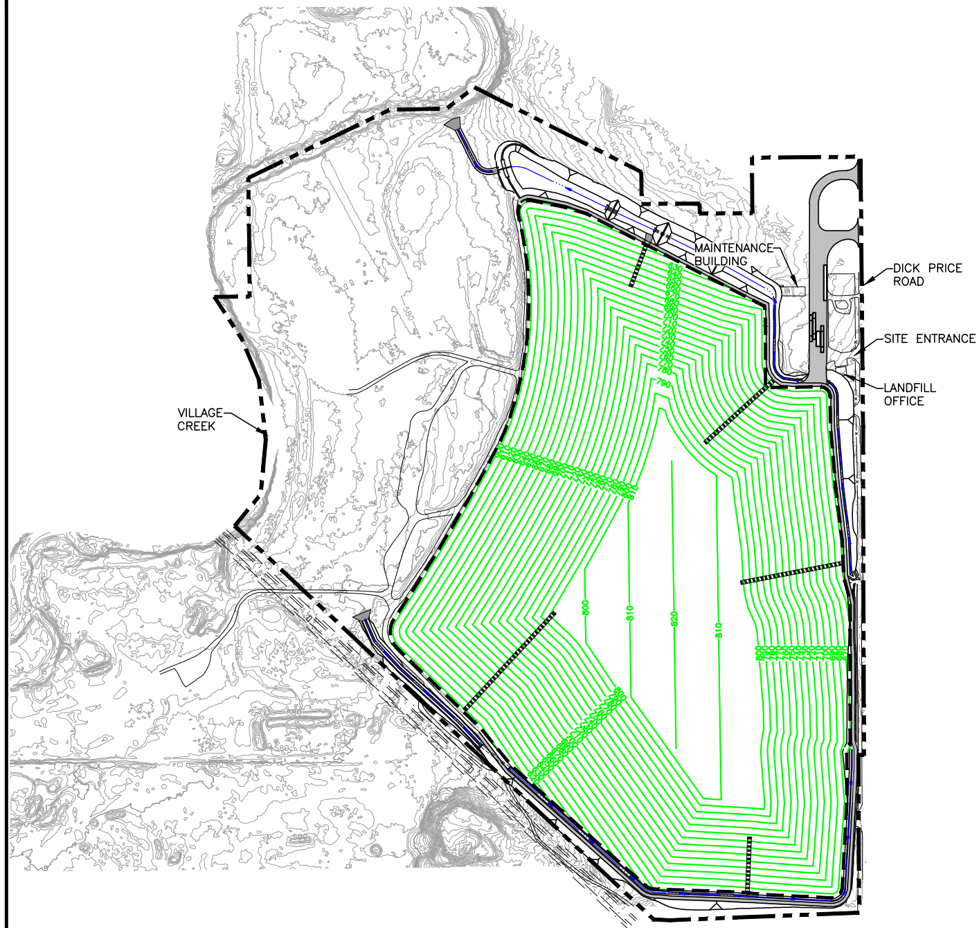
PERMITTED LANDFILL COMPLETION PLAN
